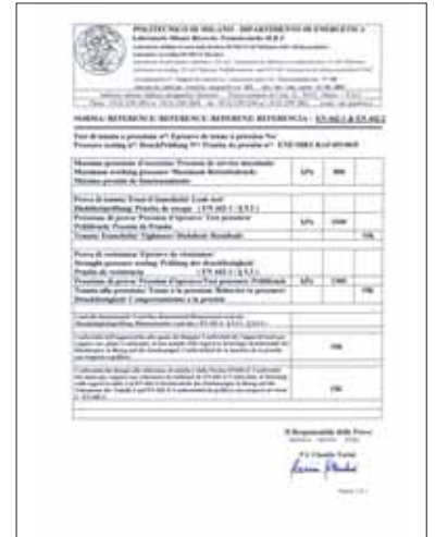
TEST REPORT Certificate of Laboratory MRT (Politecnico di Milano-Italy) on following tests: hydraulic pressure test, maximal operating pressure, endurance and conformity of radiator to the drawing's dimensions according to the standard EN 442-1 e EN 442-2.
